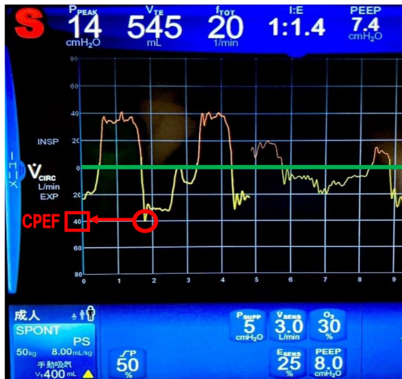
Fig. 2 How to read graphic waveforms. Graphic waveform of flow rate-time. The vertical axis represents the flow rate (L/min), whereas the horizontal axis depicts time (seconds). The green line shows the baseline, and below the baseline is the exhalation. The maximum flow rate of exhaled air was visually read from the graph and used as data
