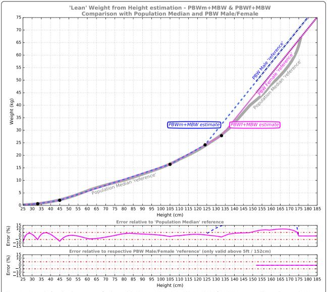
**Fig. 2** 'Lean' weight from height estimation for the models PBWm + MBW (*dashed blue*) and PBWf + MBW (*magenta*). These adhere to the Devine PBW references [19] (shown dotted) where viable, but at smaller statures adopt a unisex extension targeting the Population Median reference (shown in grey). Shown underneath is the error performance for the model relative to the respective reference curves (male – *blue*, female – *magenta*)
