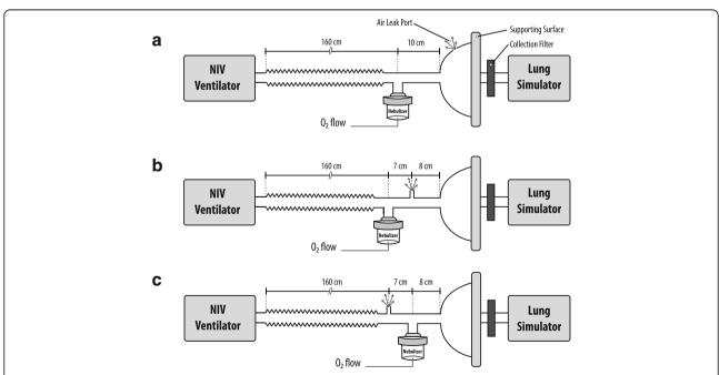
**Fig. 1** Experimental settings, see text for detailed explanation. Configuration **a**: leak port included in the vented mask; Configuration **b**: leak port between the nebulizer and the unvented mask; Configuration **c**: leak port between the nebulizer and the respiratory circuit
