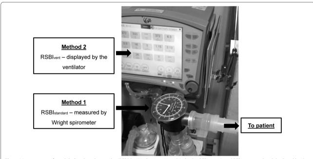
Fig. 1 Measurement of rapid shallow breathing index (RSBI) by Wright spirometer (Method 1; RSBI<sub>standard</sub>), and RSBI measured and displayed by the ventilator (Method 2; RSBI<sub>vent</sub>)
